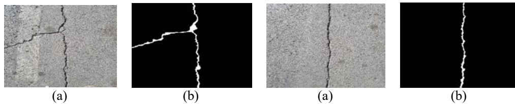
Figure 4. Dataset images; (a) The source image; (b) The ground truth images.
