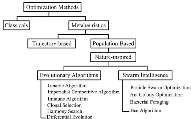
Figure 2. Metaheuristics Optimization Methods Classification [29]
